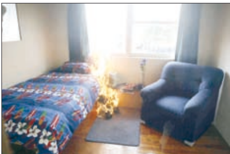
A full scale house burn demonstrates the effect of home sprinklers. Two identically-furnished rooms were set up with a small fire in a wastepaper basket. This room pictured just before the sprinkler operated.
