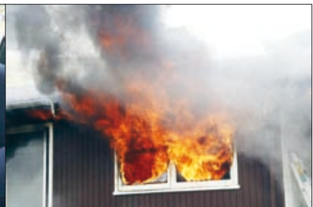
In the unsprinklered room the fire progresses to flashover, and main structural timbers have been destroyed, and the building demolished. Photographs courtesy of New Zealand Fire Service.
